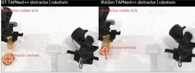
Figure S4: Representative Task 4 TAPNext++ tracking views for spatial-proximity and distractor-object interventions. Query points and tracked centroids are overlaid on simulator-reference and generated frames.
